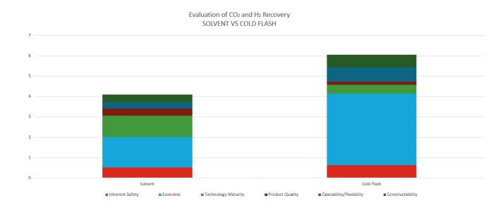
From this graph it can be concluded that the cold flash technology with PSA is the preferred technology for  $CO_2$  and  $H_2$  recovery.
