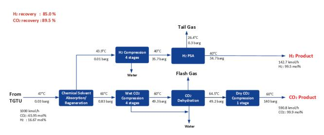
A simplified block flow diagram for the chemical absorption option is provided below:
